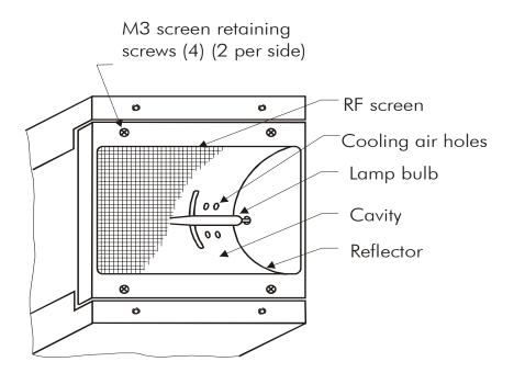
Figure 2. Reflector Assembly
